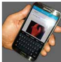
Figure 1. The WoundTool™ consists of a mobile application for image capture, a browser element for review and analysis, and a server system for data management.
